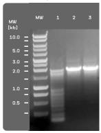
PCR amplification using ON Taq Master Mix. A 2 kb amplicon of the human beta-globin gene was amplified using onTaq PCR Master Mix (2x).
