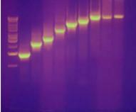
PCR amplification using EURx Perpetual *Taq* DNA Polymerase. Lane M: molecular size marker - Perfect 1 kb DNA Ladder. Lanes 0.5 to 9.3 kb: PCR amplification reactions, using Pol Buffer B with 0.2 mM dNTPs and 1.25 U EURx Perpetual *Taq* DNA Polymerase in 50 µl reaction volume.
